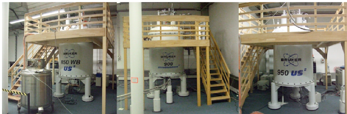
Figure 1: DFG-funded highest field NMR spectrometers. (left) 850 MHz wide-bore NMR spectrometer with facilities for magic angle spinning (MAS) low-temperature NMR experiments, (middle) worldwide 3 rd 900 MHz liquid-state NMR spectrometer, (right) world 1 st 950 MHz ultrashielded NMR spectrometer.
